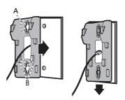
3. Align and place the telephone base on the wall mount bracket. Slide it down until it clicks securely in place.
